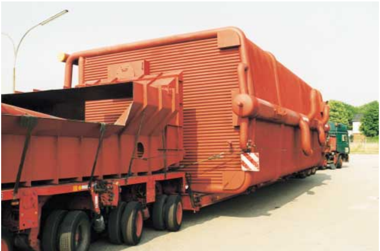
Fig. 2: 100 MW hot water - water tube boiler during transport
