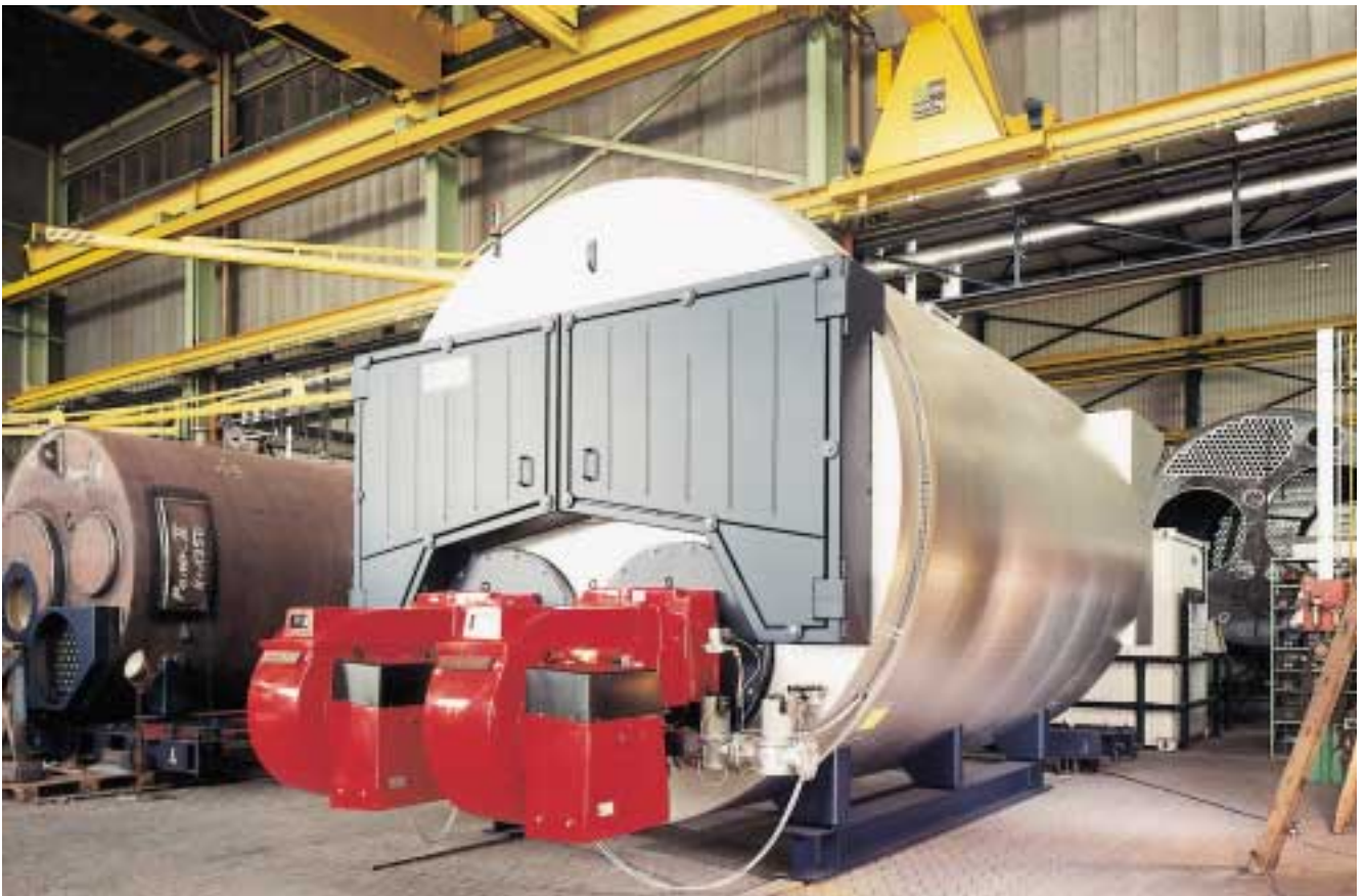
Fig. 1: High-pressure shell boiler, twin-furnace design, 35 t/h, 16 bar (make: LOOS INTERNATIONAL)
